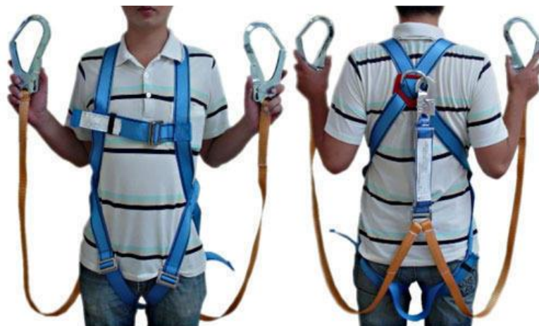
Figure 1: A full body safety harness with a shock absorber and a double lanyard
