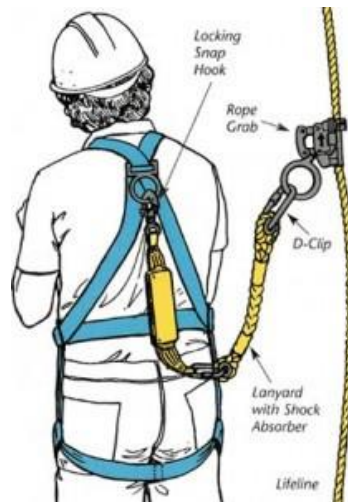
Figure 2: Safety harness with a shock absorber and a lanyard connected to the lifeline and a movable rope grab device
